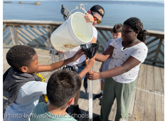
(Right) Students helping station leader hold up a turbidity tube while it is being filled with river water
